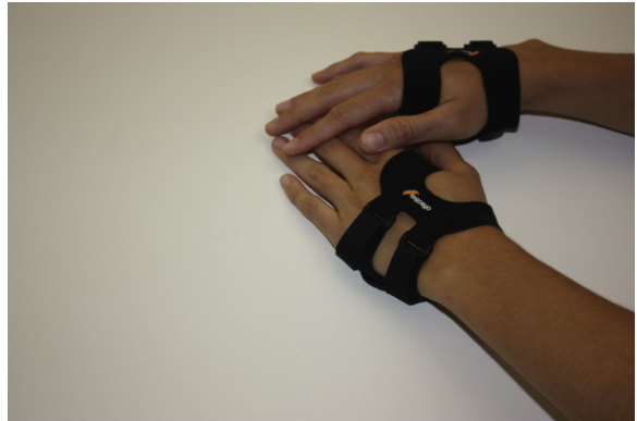
Figure 7.12 Affectiva's Q Sensor, a wearable, wireless biosensor.
